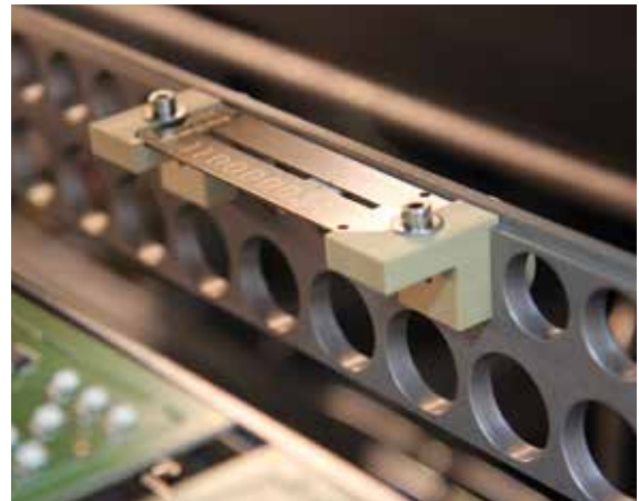
Workpiece carrier with temperature sensor in the loading position
