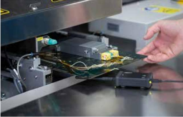
Measurement with data logger
