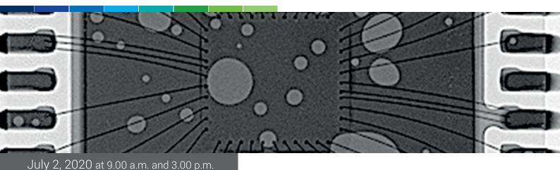
Vacuum soldering has been a proven technique for decades in contactheat and vapour phase soldering systems, significantly reducing gasbubbles in solder joints. What does this mean in terms of convection soldering, though, the most widely used and highest-throughput soldering technique today?
