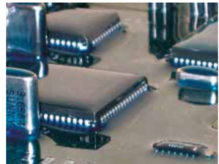
Drying process for protective lacquer coating
