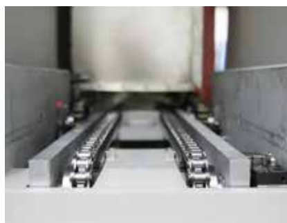
Inlet transport in a lowered position
