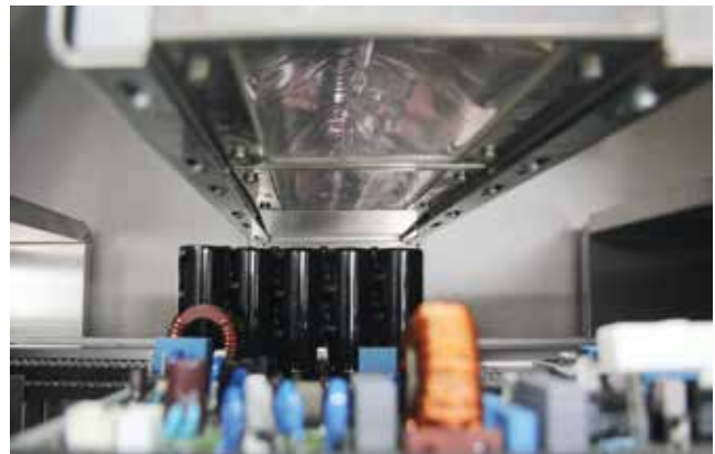
High-performance lamps in the RDS UV system dry all types of UV coating
