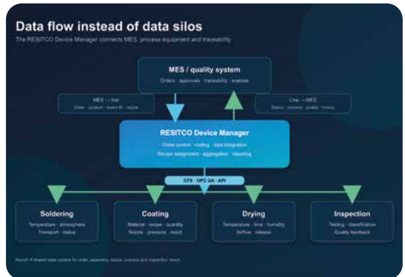
Fig. 1: Horizontal board flow and vertical data exchange in a connected production line.
